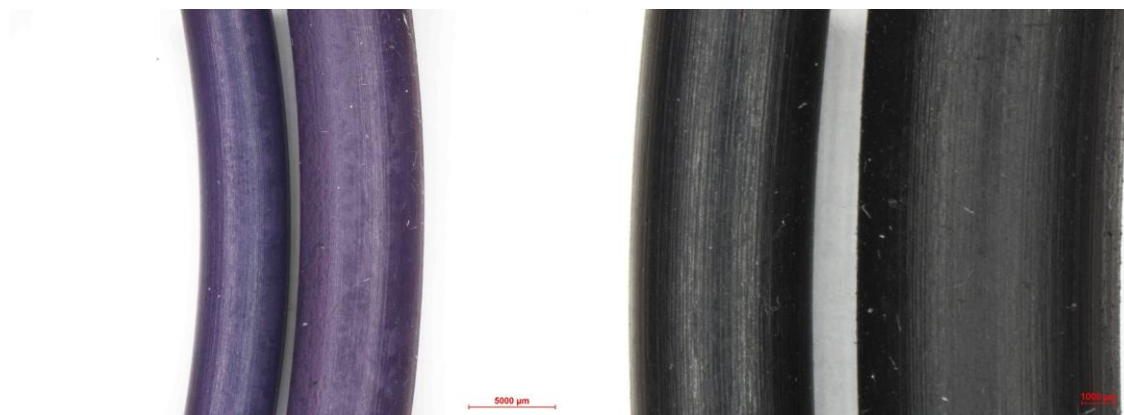
Figure 1. Example of swelling observed in EPDM (left) and IIR (right) after exposure to R-1233zd(E)/MO. For reference, unexposed material is on the left in each photograph.
